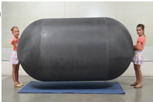
BHL™ Cryotank Validated 4X Mass Improvement
