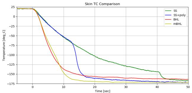
Significant change in cooling rate due to reduced heat capacity of BHL tube and polymer surface
